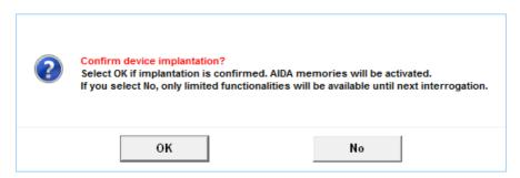
Click "No", the Overview screen will display, with the status in the header bar: "Implantation not confirmed": only some programming actions are allowed (no tests on leads, no access to AIDA memories).
