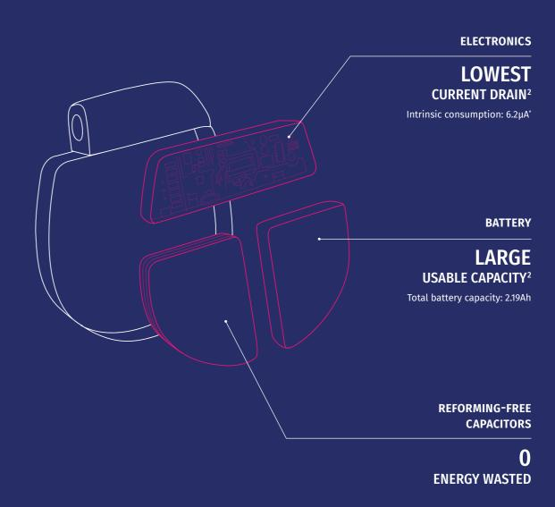
MicroPort® CRM BLE ICD and CRT-D incorporate advanced technology that withstands the test of time. With the lowest current drain and a large battery capacity, MicroPort® CRM excels in predicted longevity by up to 50% more in comparison to devices from other manufacturers.<sup>1,2</sup>
